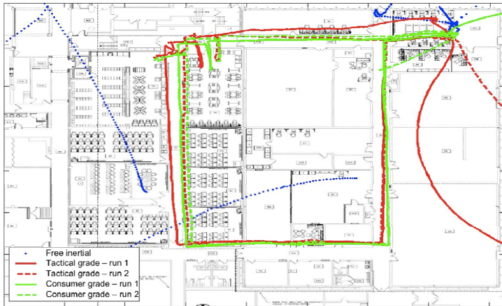
Figure 6: Results of the image-aided inertial navigator using tactical and navigation grade IMUs.
